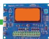
P/N - CM796B Wiegand to DF RS485 LAN Interface Module F.01U.287.314
